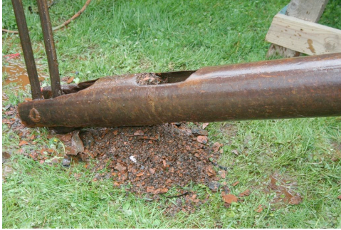
Figure 2: Bailer used for removing debris from the wells.
