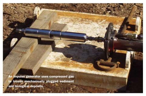
zone, and, through a pressurized hose, temporal impulses of high-pressure nitrogen are released. The impulse generator is equipped with a valve system that releases the accumulated energy (200 psi to 1,200 psi) in millisecond bursts through a large cross-sectional area.
