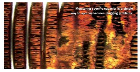
plugging is occurring and if rehabilitation is necessary. A periodic pumping test will help determine if the well has lost efficiency, which—if there's no biological plugging—could indicate mechanical plugging from the migration of fines.
