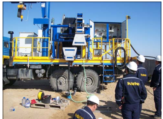
Photo: hydrolift operation in Kazakhstan parallel or after pulsing with hydropuls ® - process. Special development of TLM hydropuls GmbH for JV Katco (Areva-Kazatomprom)
