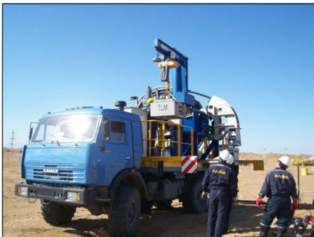
Photo: hydrolift operation in Kazakhstan parallel or after pulsing with hydropuls ® - process. Special development of TLM hydropuls GmbH for JV Katco (Areva-Kazatomprom)
